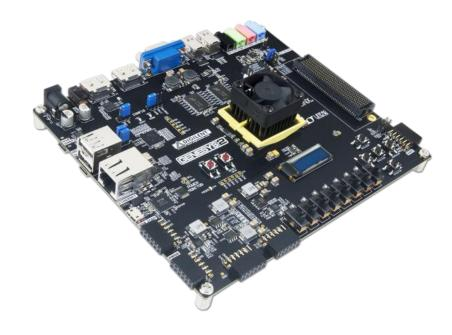
**RiscFree** Eclipse based IDE + Opella-XD JTAG Probe + Genesys2 FPGA Board
